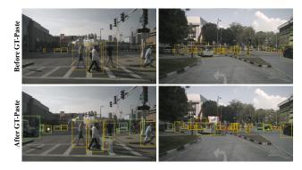
Figure 6. Qualitative results of 2D detection after our data augmentation. Top row: 2D detection results of original scenes. Bottom row: the results after our GT-Paste data augmentation. Yellow and green boxes respectively denote the detection results of original and pasted objects. Red boxes are the false negative predictions.
